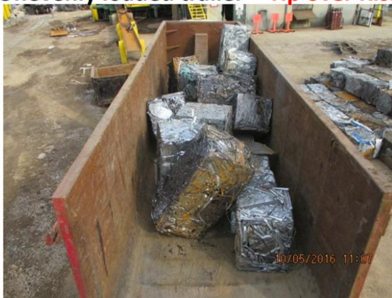
Unevenly loaded trailer – Tip over Risk
